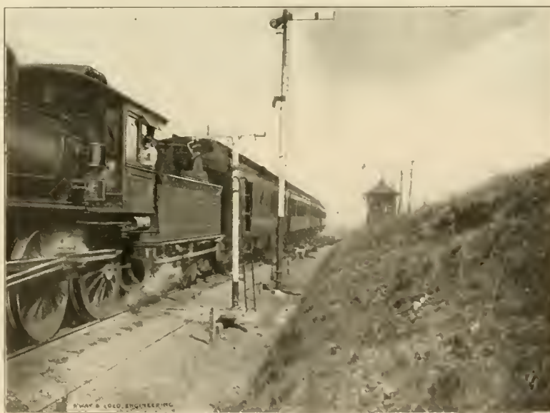
C., N. O. & T. P. TRAIN IN THE ACT OF CATCHING STAFF.
